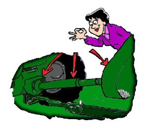
All PTO shields should be in place and in good working condition.
