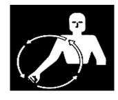
**START THE ENGINE**--Simulate cranking of vehicles by moving arm in a circular motion at waist level.
