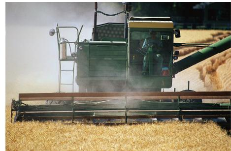
The combine cuts off the heads of the plants, shakes the wheat kernels out of the heads, and separates the kernels from all the other plant materials. The kernels are moved into a grain tank on the combine. All the extra plant material is blown out of the back of the combine and spread across the field. When the grain tank on the combine is full, the grain is deposited into a truck that drives the wheat to a grain elevator for storage.
